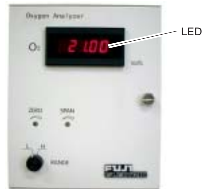
Turning on the power lights up the measurement LED.
